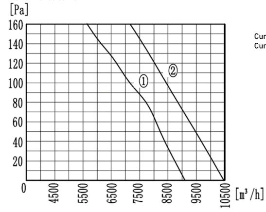
Curve 1: 50HZ Curve 2: 60HZ
